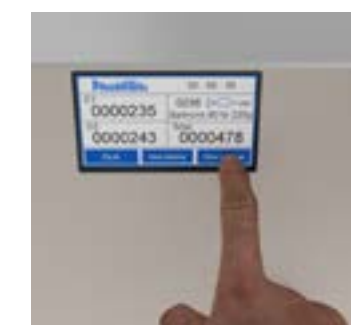
A large touch screen allows to check the counter and to display information.
